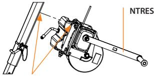
Fit the locking pin into the hole in the tripod leg
